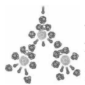
Procedure of releasing the nuclear energy. Uncontrolled process is called atomic bomb, and controlled process is a nuclear reactor.
