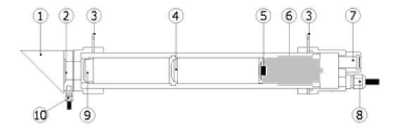
(1) protection cap, (2) window with heater, (3) sight, (4) aperture tube,(5) sensor, (6) thermopile, (7) humidity indicator, (8) cable gland, (9) window assembly with heater,(10) cable for heater.
